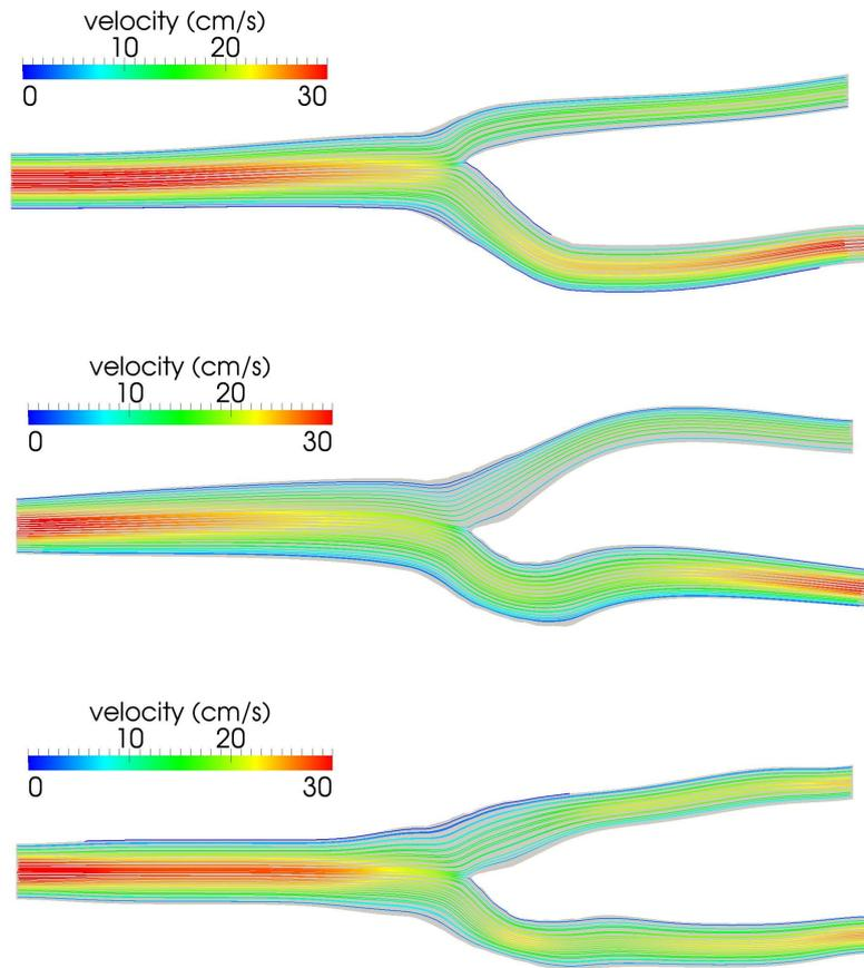
**Fig. 4.** Optimal configuration obtained by minimizing the viscous energy dissipation for the FFD case (top), the RBF case with the thin-plate spline option (middle) and the RBF case with the Gaussian option (bottom)
